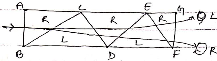
ABFG = a rectangular block made of alternate prisms of right-handed & left-handed quartz, all having their optic axis  $\perp$  to end faces AB & FG.
