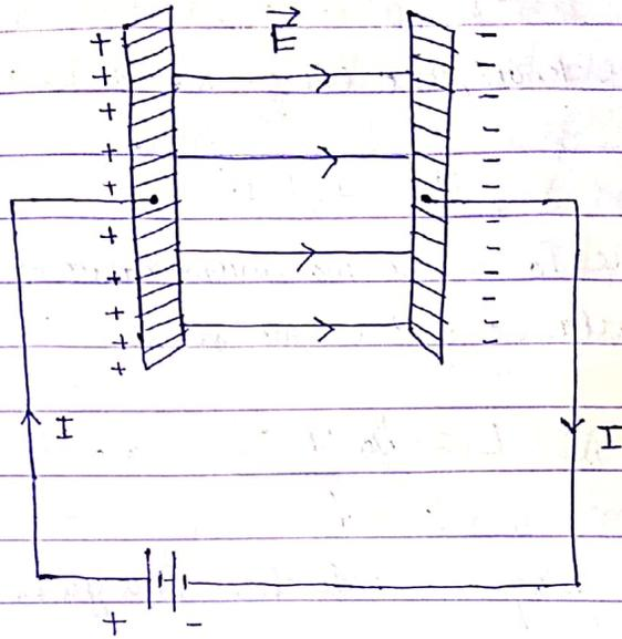
Maxwell showed that Kirchoff's law can be obeyed by this circuit <sup>having a capacitor</sup> if some sort of current is associated in the gap of the plates of the capacitor.
