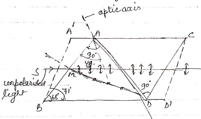
It consists of a calcite crystal AB whose length is about three times of its width. Its end faces AB and CD are cut such that angles of principal section becomes 68° and 112° instead of 71° & 109°.
