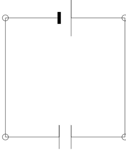
FIG. 24: Schematic representation of a capacitor and a battery. The short fat terminal is negative. The capacitor acquires the same voltage  $V$  as between the terminals of the battery. The charge taken by the capacitor is  $Q = CV$ . If disconnected from the battery, the capacitor will keep this charge.
