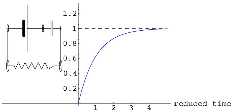
Charging a capacitor. Reduced time is  $t/\tau$ ; reduced charge and voltage are  $q/\mathcal{E}C$  and  $V/\mathcal{E}$ , respectively. Current follows a decay exponential, as in Fig. 33.
