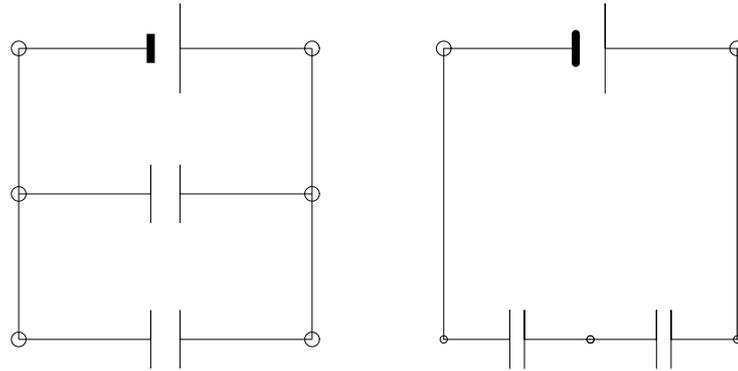
FIG. 25: Parallel (left) and series (right) connections. If each pair of the capacitors will be replaced by a single equivalent capacitance, as in Fig. 24, with the values of  $C_{eq}$  given by eq. (48) or eq. (49), the battery will "not know" about the change. In particular, the total charge taken from the battery will be  $Q = C_{eq}V$ , the energy stored will be  $(1/2)V^2C_{eq}$ , etc.
