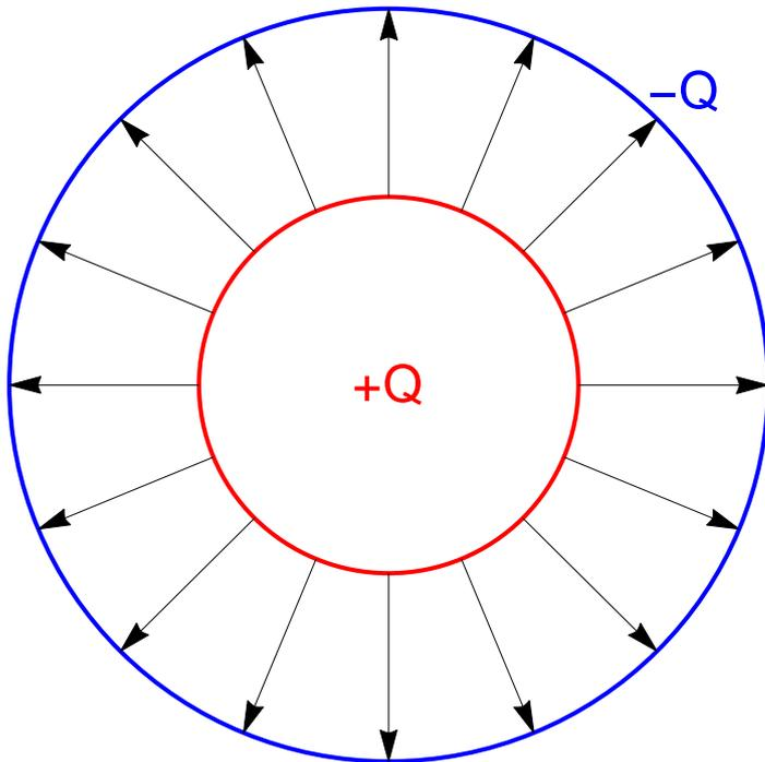
Let us surround the inner sphere (radius  $R_1$ ) by a larger thin spherical shell with radius  $R_2$ . The charge  $Q$  is placed on the inner sphere, and the charge  $-Q$  on the outer one. The field is now given by
