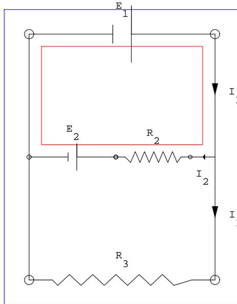
FIG. 32: Example of a two-loop circuit
