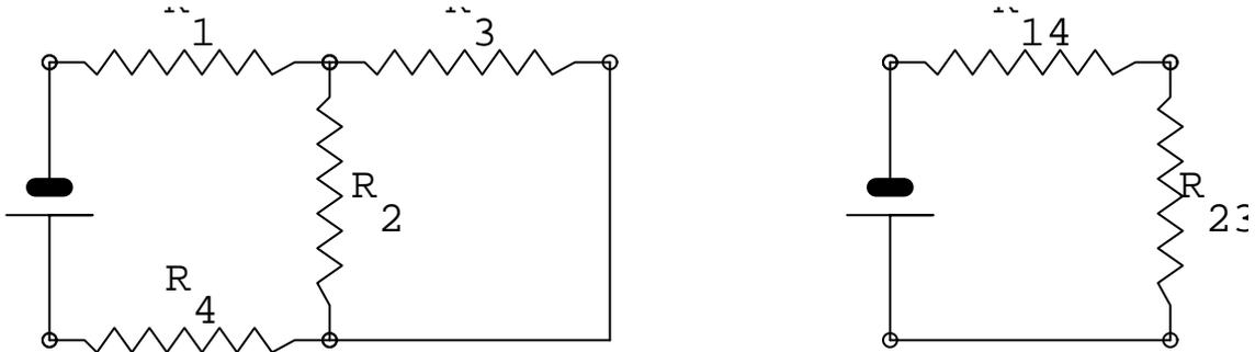
FIG. 28: Example of the reduction method
