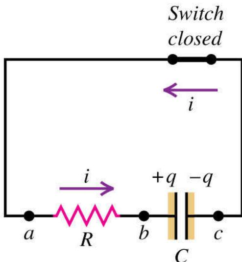
When the switch is closed, the charge on the capacitor and the current both decrease over time.
