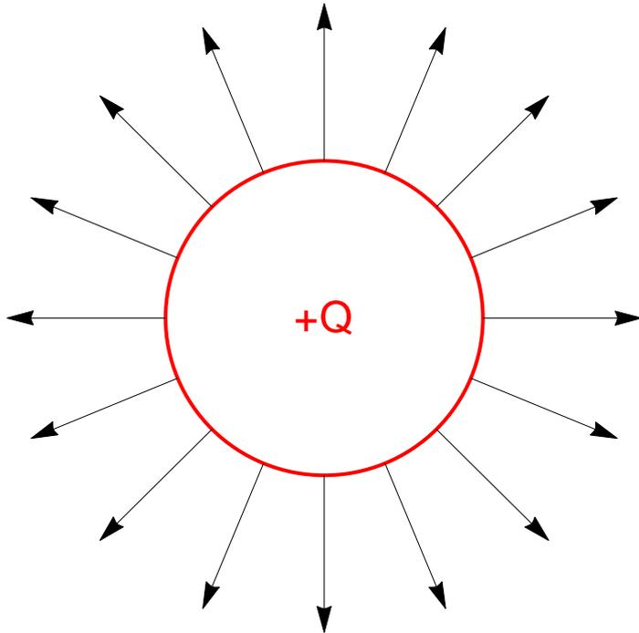
Consider a conducting sphere with radius  $R$ . To find  $C$  we place on it a charge  $Q$  and find  $V$ .
