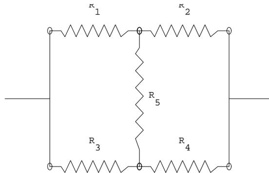
FIG. 29: Irreducible circuit
