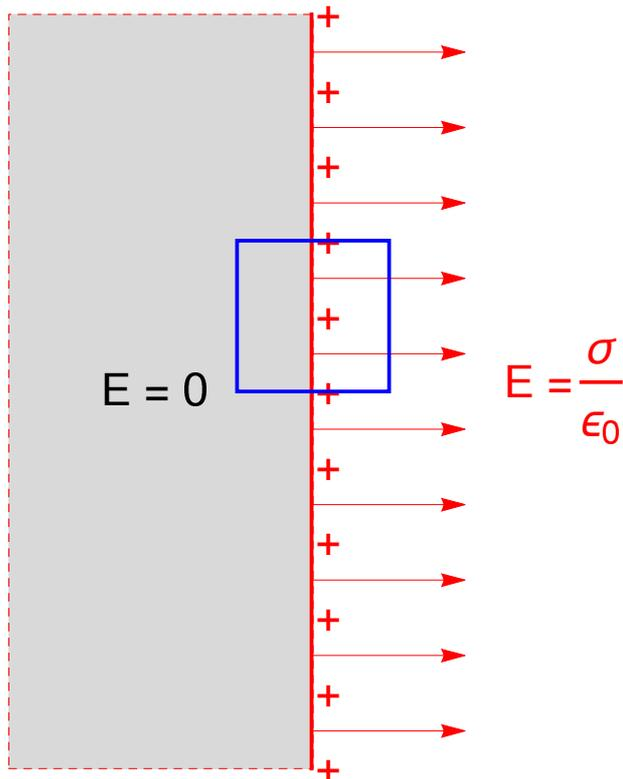
Field is now 'one-sided' (compare with fig. 19 for an insulator). For a conductor, Gauss theorem gives
