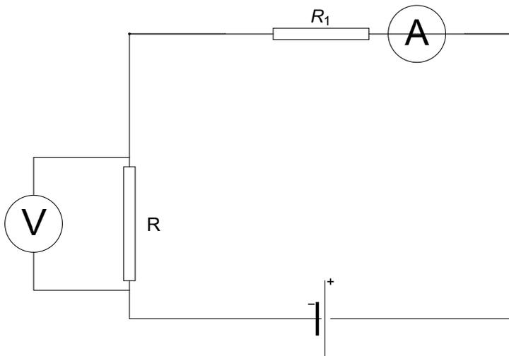
ammeter - in series with resistor,  $R_A \approx 0$  ("ideal ammeter",  $R_1 + R_A \approx R_1$ )
