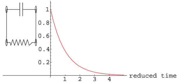
FIG. 33: Discharging a capacitor. Reduced time is  $t/\tau$ , with  $\tau = RC$ . Reduced charge, voltage, current are  $q/Q_0$ ,  $V/V_0$  or  $i/i_0$ , respectively, with  $V_0 = Q_0/C$  and  $i_0 = -V_0/R$ .
