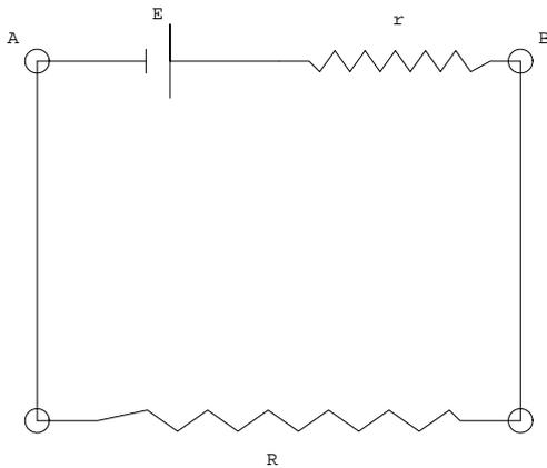
The real battery.  $R$  is the external load,  $r$  is the internal resistance. Find the voltage between the terminals  $A$  and  $B$ .
