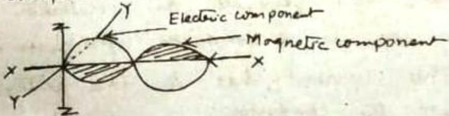
When microwave is irradiated on a substance (dipole) having dipole moment then its dipole tries to reorient itself with the alternating electric field component of radiation, & it loses its energy in the form of heat by molecular friction.
