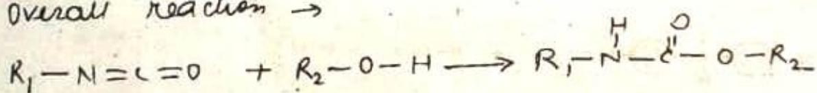
The use of  $\text{CO}_2$  gas formed in step (ii) is for making foam (cells). However this reaction may be replaced by using a volatile liquid e.g. n-pentane.
