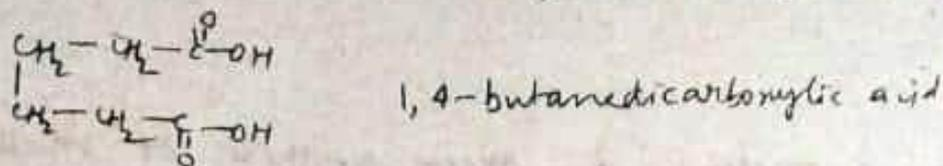
It occurs in nature in a very small amount. From industrial point of view, it is most important dicarboxylic acid. It is mainly used for production of nylon. It is white crystalline powder (m.p = 152°C)
